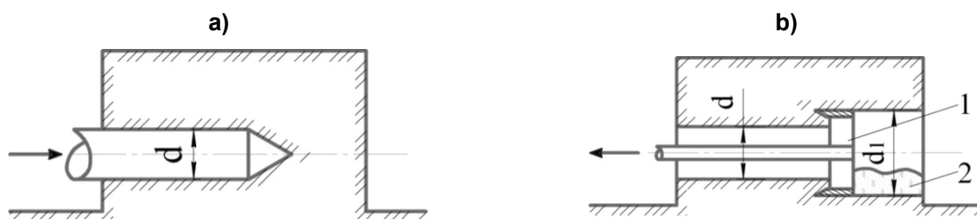
Figure 3. Scheme of the well expansion with a cutting ring: a – pilot thrust boring; b – well expansion with a cutting ring 1 – cutting ring; 2 – cut soil
