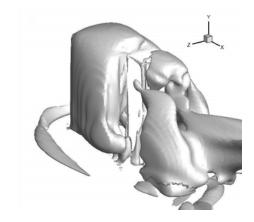
Figure 1. Model of building ensemble in a wind tunnel (a), failure of a vortical veil at a flow of a tandem of buildings (b) and comparison settlement and experimental *Cp* on the back side of the second building (c)
